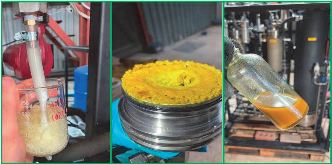
Figure 2b. Final products of SCF separation of various components of plant raw materials.
